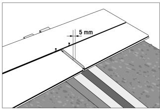
Exclusively use Cobra® clips and screws from FIBERDECK®. This is mandatory for the warranty to remain in effect. These clips ensure good spacing between boards placed side by side.
