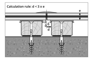
Do not block air circulation under the board.
