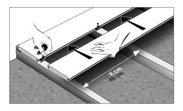
1 - First, fasten the starting clips on the joist, then insert the first board.2 - Insert the clips in the groove of each joist.
