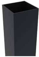
Reinforced sealing post with 90x90mm section. Thickness 4mm Associated with profile Ref. 1278, it allows the wicket to be inserted into the fence without an additional post
